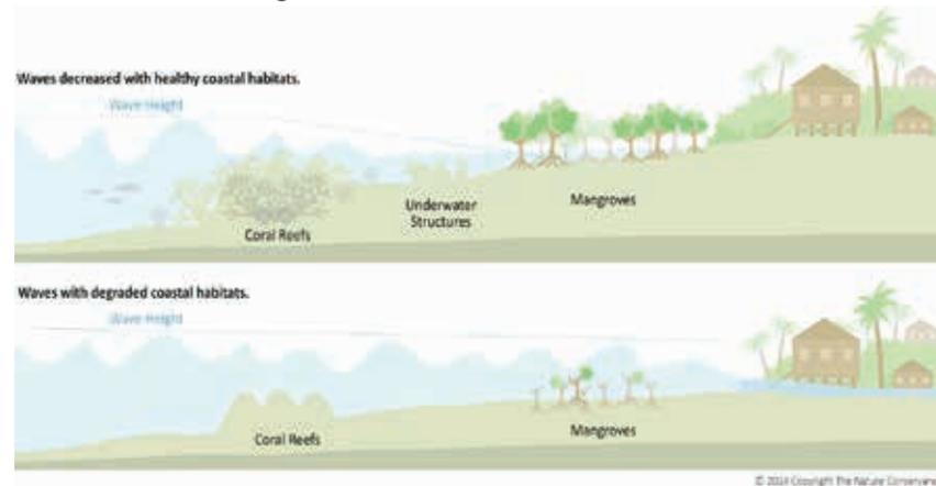
**Natural coastal defense.** The upper image illustrates how the complex structures of coral reefs, mangroves and other ecosystems can play an important role in reducing wave heights and protecting communities. When degraded or lost (lower image) this capacity to reduce waves is greatly diminished and the threat of flooding and erosion increases.
